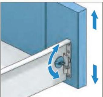
Adjust the drawer frontal height by rotating the lever clockwise/anti-clockwise.
