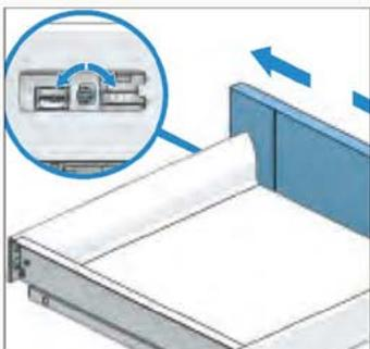
To adjust the drawer front vertically clip off the cap, rotate the grooved wheel clockwise/anti-clockwise.
